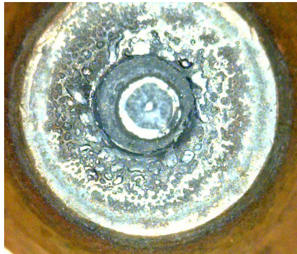
Figure 60 – Non-symmetrical, rough-edged pit and rough-surfaced electrode face
