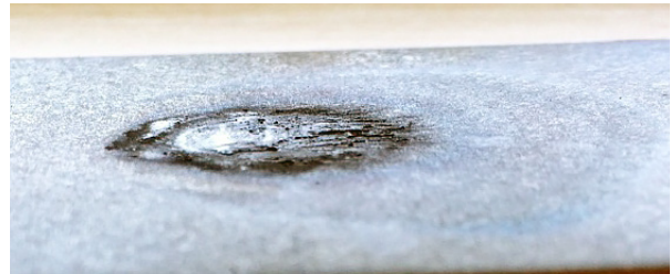
Spot weld removed
